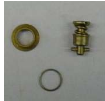
A1690 Camlock Stud, Grommet and Snap Ring for AA1 Upper Forward Cowling Attachment
