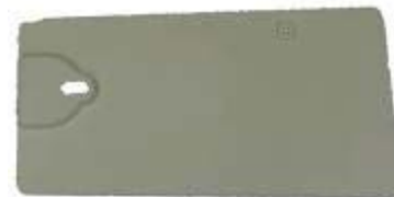
5102353-7 Plastic overlay for baggage door
